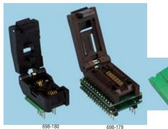
To assist with product development, the following adaptors have been designed for use with the PICSTART Plus programmer.
