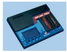
The MPLAB® PM3 Universal Device Programmer is easy to use and operates with a PC or as a stand-alone unit, and programs Microchip's entire line of PICmicro® devices as well as the latest dsPIC30F DSC devices.
