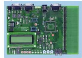
The dsPICDEM® 1.1 General Purpose Demonstration Board provides the application designer with a low-cost development solution to become familiar with the dsPIC30F 16-bit DSC architecture. The development board serves as an ideal prototyping tool to quickly develop and validate key design requirements.
